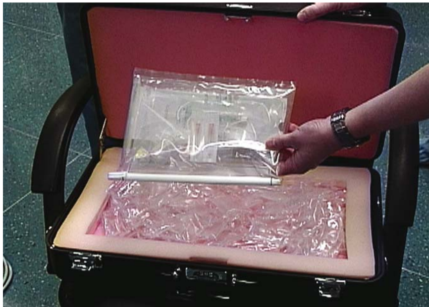
FIGURE 2. Photograph of transport case containing sterile, 30-ml cell bag packed in frozen gel packs.
